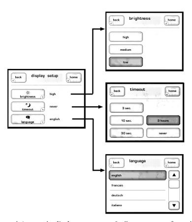
This button brings up the **display setup** menu. It allows you to configure the CP-500's LCD screen *brightness*, the display *timeout*, and the *language* used in the touchscreen and menu system.
